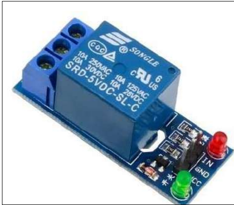
Fig 5: Image of Relay module
