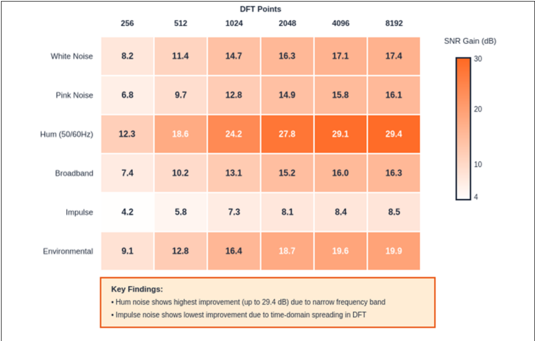
Fig 1: Heat map showing SNR improvement in dB as function of noise type and DFT window size
